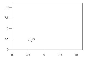
Now, let's imagine that this point (3, 2) represents a force in a certain direction. For example, we can draw a line from the origin to this point and the resulting force's magnitude will be represented by the length of the line in question (which can be obtained via the pythagorean theorem), and the direction of the force will be outwards from the origin following the line.
